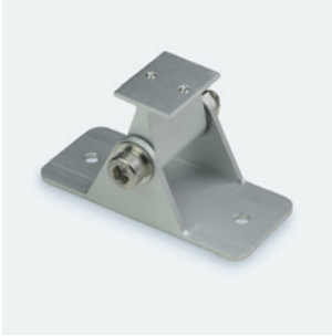
KKBK-16 Small adjustable bracket (allow 2 per metre/40in) Silver anodised aluminium finish L46/W70/H89.2mm (L1.8/W2.76/H3.51")
